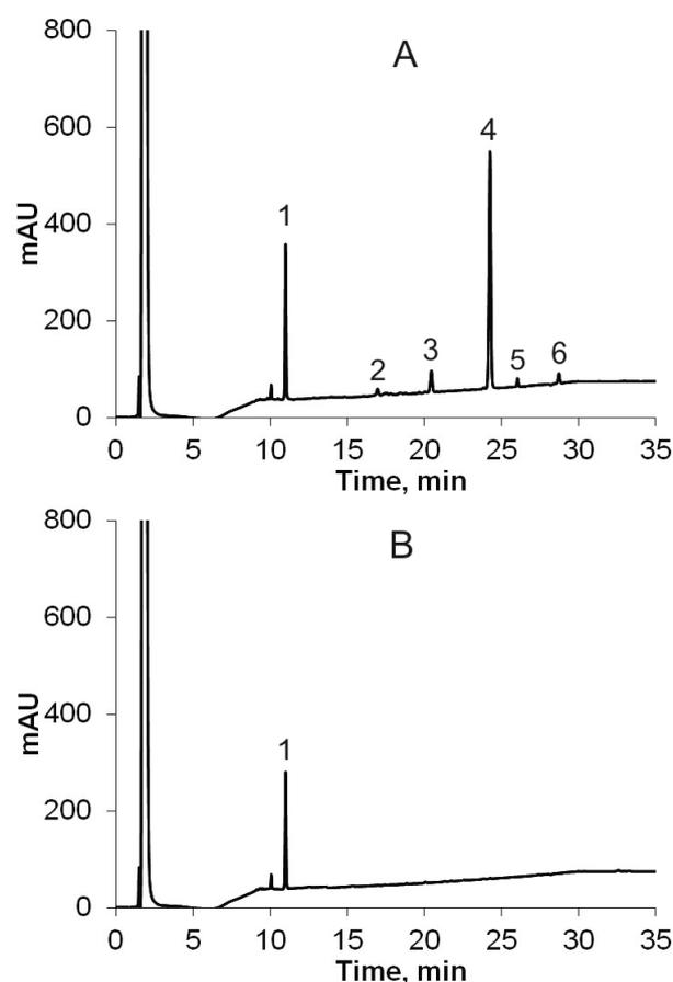
Fig. 3. HPLC-UV chromatograms (250 nm) of acetone extracts of *Sporodophoron gossypinum* (A) and *S. primorskiense* (B): 1 – lepralic high unknown; 2 – 4-O-methylolivetolcarboxylic acid; 3 – confluentic acid; 4 – 2'-O-methylperlatolic acid; 5 – perlatolic acid; 6 – hyperlatolic acid.
